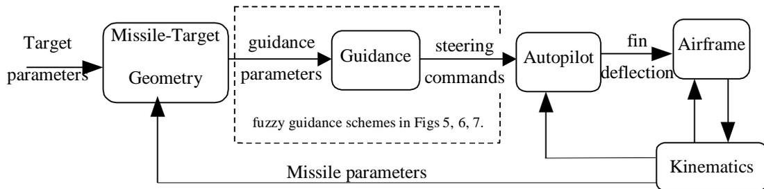
Fig. 8 Simplified block diagram of the main simulation model modules.
