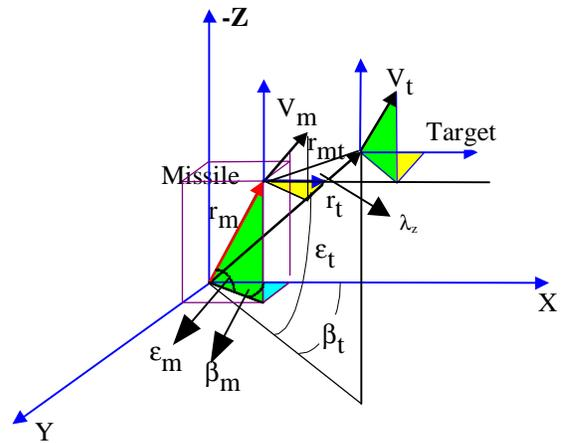
Fig. 4 Geometry of Missile-Target interception
