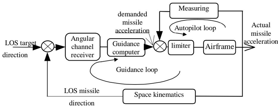
Fig. 1 Block diagram of the guidance-autopilot loop
