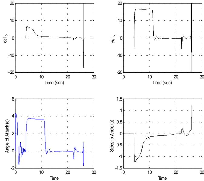
Fig. 13 Pitch and yaw control fin deflection and corresponding  $\alpha$  and  $\beta$  in case of employing FSG.
