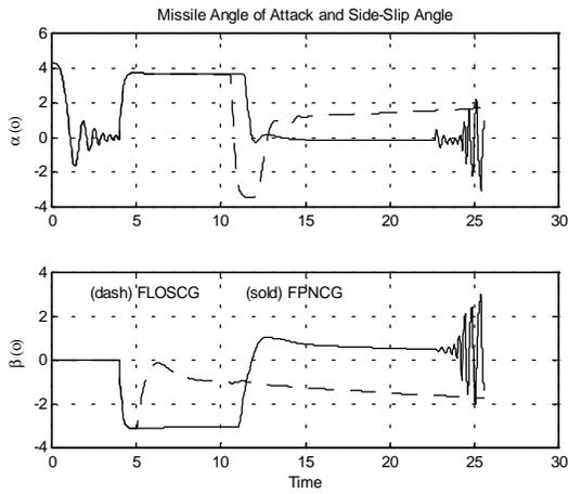
Fig. 11 Missile angle of attack and sideslip angle.
