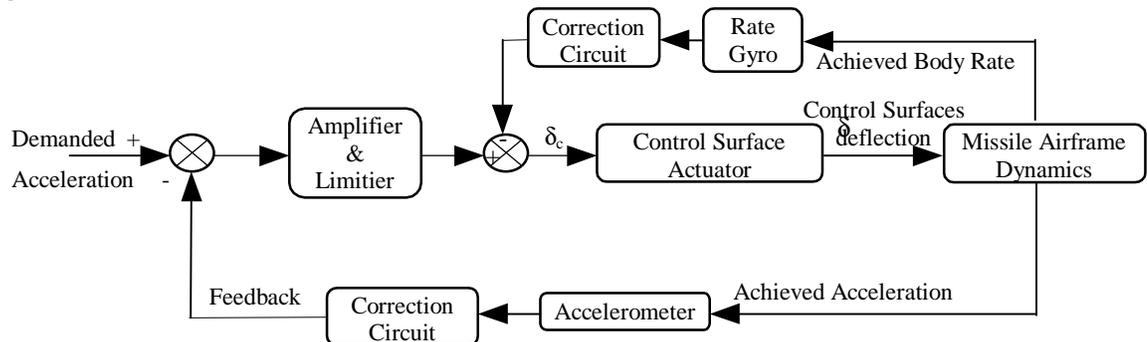
Fig. 3 Simplified block diagram of pitch autopilot.
