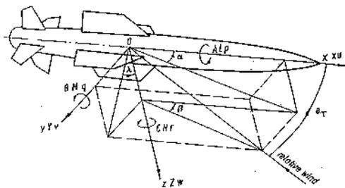
Fig. 2 Missile airframe reference axes
