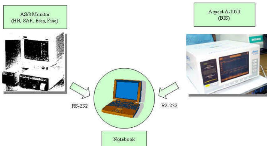
Fig. 3. An IBM compatible notebook for data acquisition of clinical data using serial communication RS232 in the operating theatre
