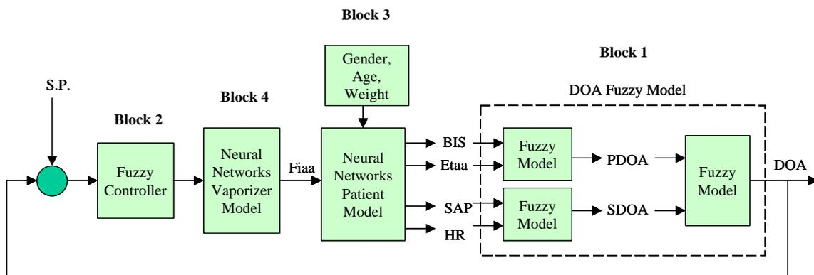
Fig. 1. A hierarchical architecture included four blocks for anaesthesia simulation during inhalation
