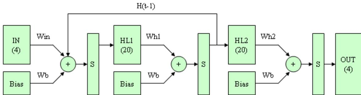
Fig. 2. A four-layer artificial neural network with one input layer having five input nodes and twenty-one recurrent nodes, two hidden layers having each twenty hidden nodes and one bias node, and one output layer having four output nodes
