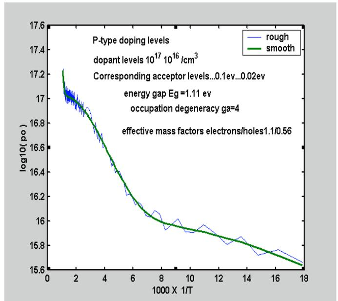
Figure 5 Multiple dopant test of numerical algorithm for which analytic model does not apply.
