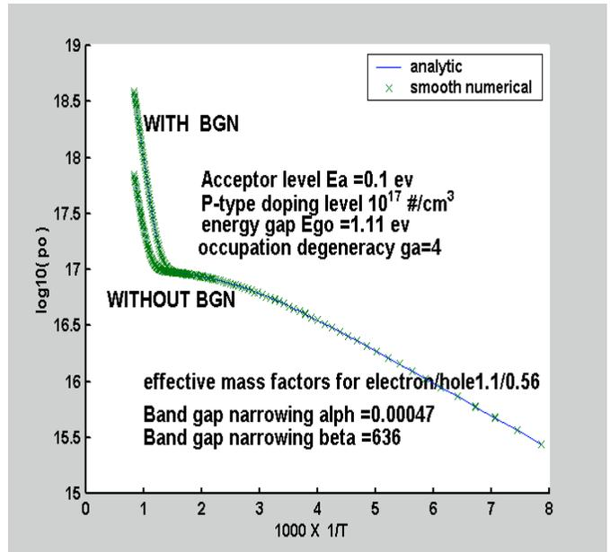
Figure 3, Comparison of analytic equation with numerical algorithm with and without band-gap narrowing (BGN).
