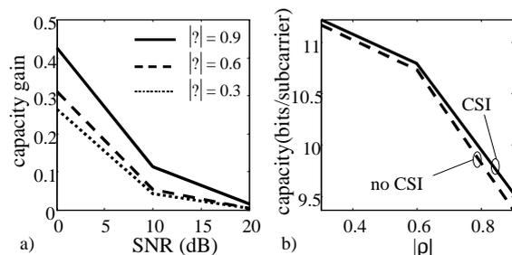
Fig.4 a) capacity gain curves for three absolute values of the correlation coefficient at only one side of the channel. b) capacity curves for 20 dB SNR with and without CSI at the transmitter.
