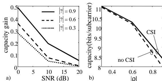
Fig.3 a) capacity gain curves for three absolute values of the correlation coefficient at both receive and transmit sides. b) capacity curves for 20 dB SNR with and without CSI at the transmitter.
