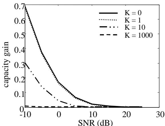
Fig.2 Capacity gain:  $(C_{\text{CSI}} - C_{\text{noCSI}}) / C_{\text{noCSI}}$ .
