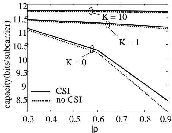
Fig.7 Capacity curves for 20 dB SNR for three different values of  $K$ . The curves correspond to the average case in figure 6 and the correlation coefficient applies to both transmit and receive side.
