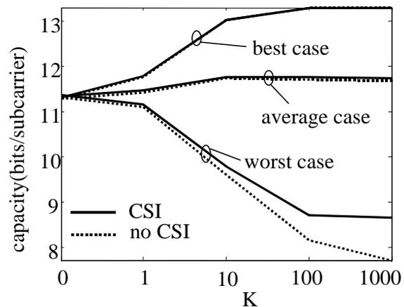
Fig.6 capacity curves for 20 dB SNR and three different choices of the phases of the entries of matrix  $\mathbf{M}$ .
