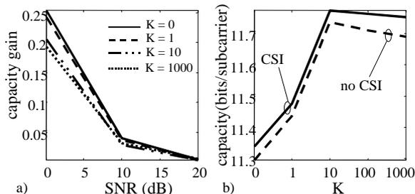
Fig.5 a) capacity gain curves for four values of factor  $K$ . No spatial correlation is assumed. b) capacity curves for 20 dB SNR with and without CSI at the transmitter.
