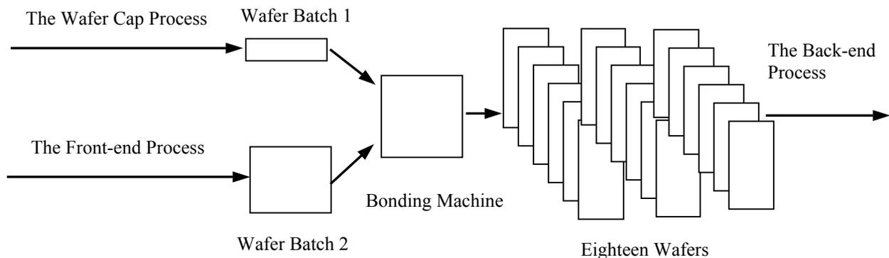
Figure 1 Schematic View of the Whole MEMS Process
