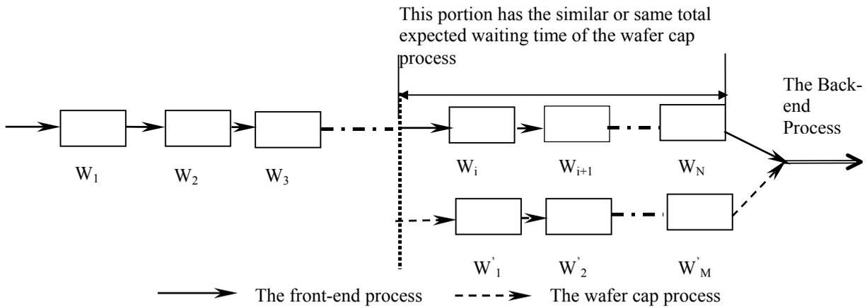
Figure 4 Schematic View of the QUEUESYN Rule and Two Virtual Flow Shops
