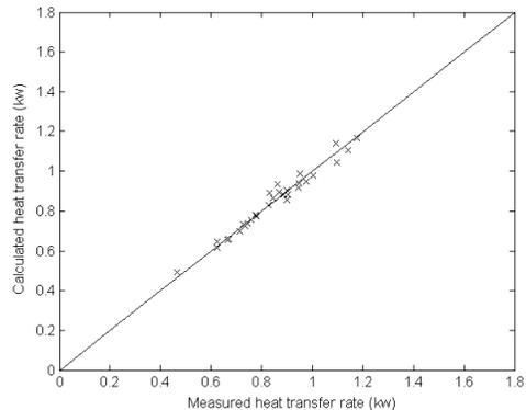
**Fig. 5** Heat transfer rate calculated versus measured for three parameters case
