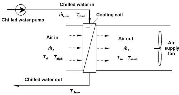
**Fig. 1** Schematic of cooling coil
