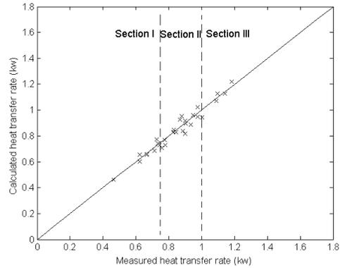
**Fig. 4** Heat transfer rate calculated versus measured for two variable parameters case
