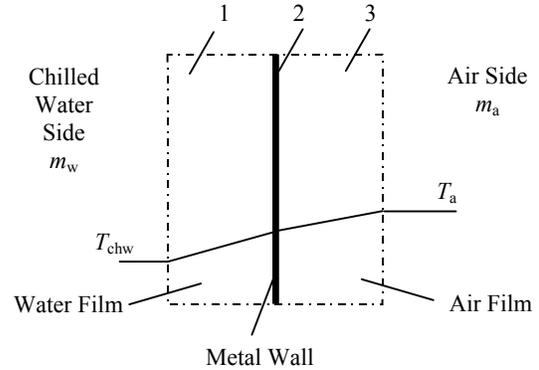
**Fig. 2** heat transfer model of coil
