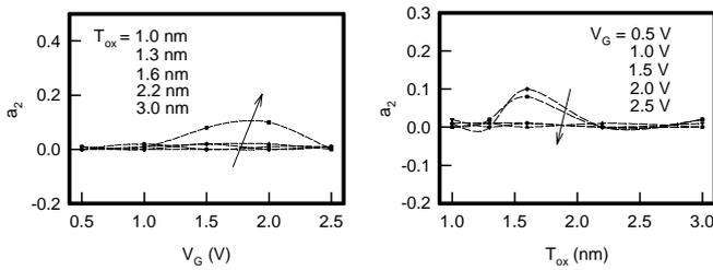
Fig. 5. (a) The plot of  $a_2$  versus  $V_G$ . (b) The plot of  $a_2$  versus  $T_{ox}$ . The  $a_2$  is set to be zero constant.
