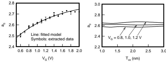
Fig. 3. (a) The plot of  $a_0$  versus  $V_G$ . (b) The plot of  $a_0$  versus  $T_{ox}$ . We note that the  $a_0$  is exponential dependence on  $V_G$  and nearly constant on  $T_{ox}$ .
