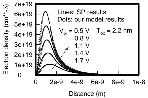
Fig. 7. The electron density distribution with the SP equations and our developed model, where the oxide thickness is fixed at 2.2 nm.
