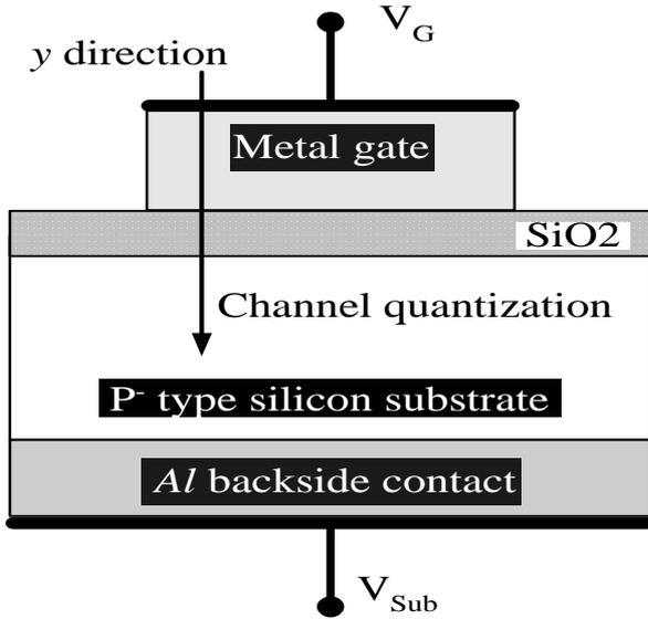
Fig. 1. A plot of 2D cross section for nanoscale N-MOS devices.
