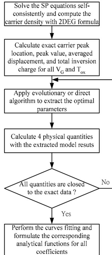
Fig. 2. An evolutionary procedure to extract the coefficients formula for the compact charge model for nanoscale N-MOS devices.
