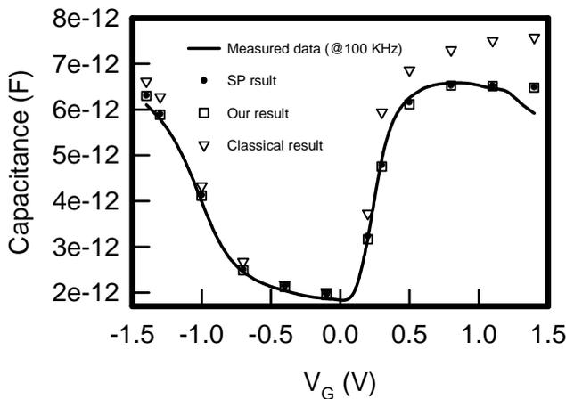
Fig. 10. A comparison of the simulated and measured C-V curves for the proposed compact model and the SP model.
