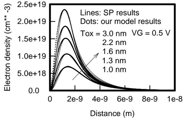
Fig. 8. The electron density distribution for different oxide thicknesses. The applied voltage is fixed at 0.5 V. The solid lines are SP results and dots are our model data.
