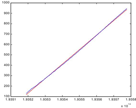
Fig.5(b) Group delay response (rippled) and linear regression for a 50 km,  $D_F=17$  ps/nm/km link, raised cosine-apodized grating ( $a=1$ )
