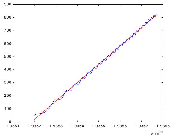
Fig.5(a) Group delay response (rippled) and linear regression for a 100 km,  $D_r=17$  ps/nm/km link, raised cosine-apodized grating ( $a=0.4$ )
