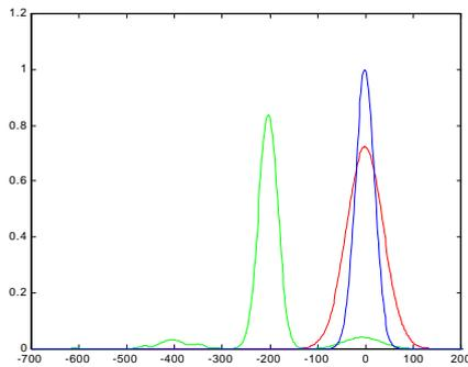
Fig.2(b) Initial, transmitted and recompressed pulse for a 50 km,  $D_f=17$  ps/nm/km link, non-apodized grating.
