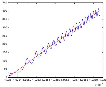
Fig2.(a) Group delay response (rippled) and linear regression for a 50 km,  $D_f=17$  ps/nm/km link, non-apodized grating
