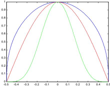
Fig 1. Raised cosine apodization profiles of increasing strength  $a=0.4$  (solid,  $a_{\text{eff}}=0.7$ ),  $a=1$  (dotted,  $a_{\text{eff}}=0.6$ ),  $a=4$  (dashed,  $a_{\text{eff}}=0.37$ )
