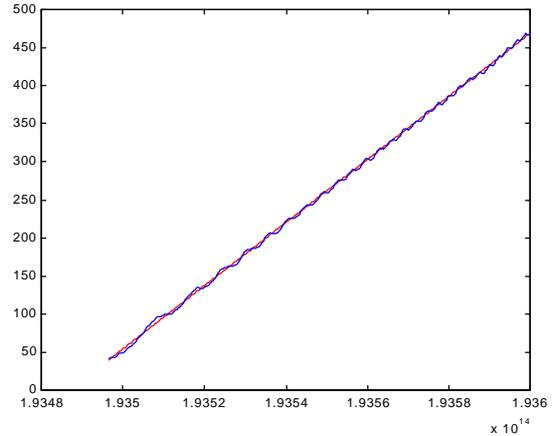
Fig.3. Group delay response (rippled) and linear regression for a 50 km,  $D_f=17$  ps/nm/km link, raised cosine-apodized grating ( $a=0.4$ )
