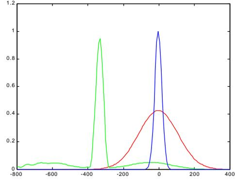
Fig 4. Initial, transmitted and recompressed pulses for a 100 km,  $D_r=17$  ps/nm/km link, non-apodized grating.
