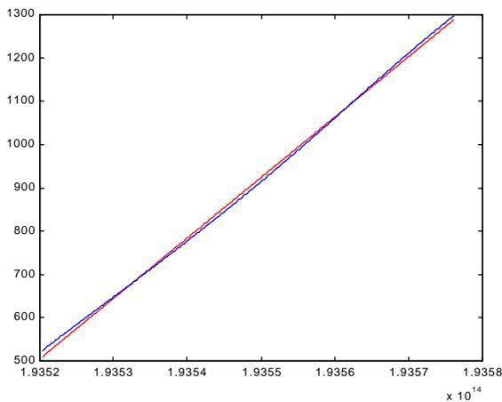
Fig 5(c) Group delay response (rippled) and linear regression for a 50 km,  $D_F=17$  ps/nm/km link, raised cosine-apodized grating ( $a=4$ )
