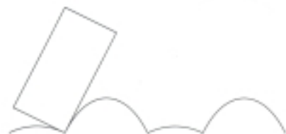
Fig. 6 – Rectangular wheel moving on a sequence of catenary arcs
