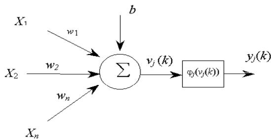
Fig. 2 - Representation of the artificial neuron.
