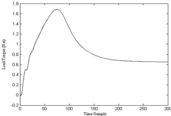
Fig. 4 - Estimation of torque to constant load.
