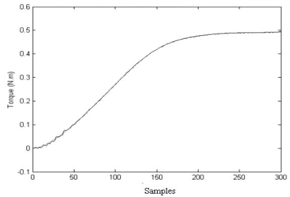
Fig. 7 - Estimation of torque to linear load.
