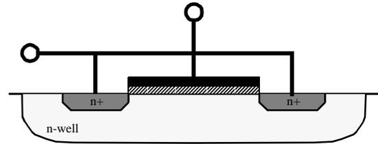
Figure 2 Accumulation mode varactor.
