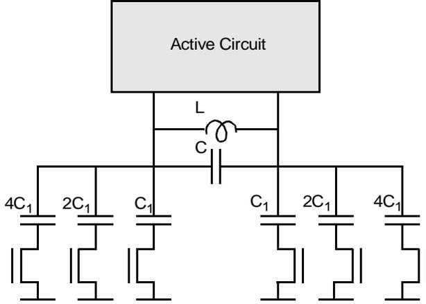
Figure 3 Binary weighted array of capacitors.
