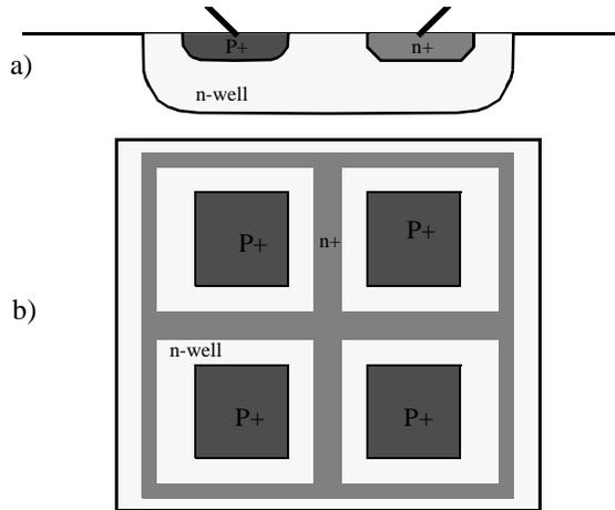
Figure 1 An  $n$ -well  $p^+$  varactor in CMOS technology.
