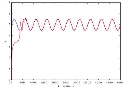
Fig. 3 Tracking of a sinusoidal setpoint by output  $y$  (solid line: actual value, dashed line: reference )
