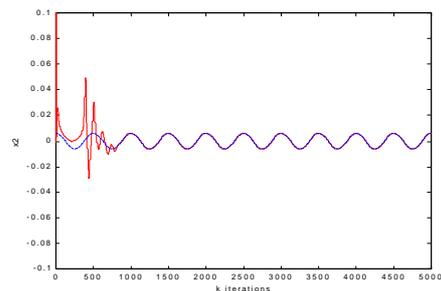
Fig. 5 State variable  $x_2$  converges to the reference signal  $x_{2\text{des}}$  (solid line : actual value, dashed line : reference )
