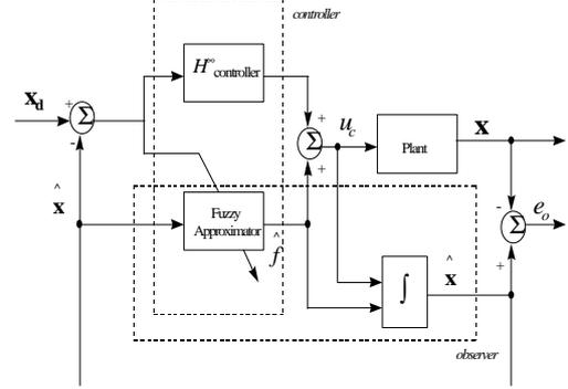
Fig. 2 The observer-based adaptive fuzzy  $H^\infty$  control architecture
