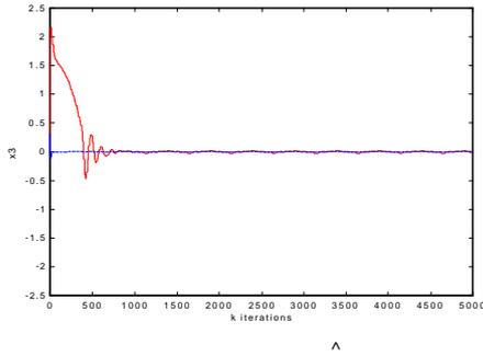
Fig. 6 Observed state variable  $x_3$  converges to the actual state variable  $x_3$  (solid line : observed state , dashed line : actual state )
