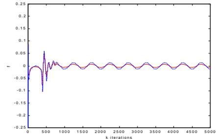
Fig 4. Estimation of parameter  $f$  by the adaptive fuzzy system (solid line :  $\hat{f}$  , dashed line  $f$  )
