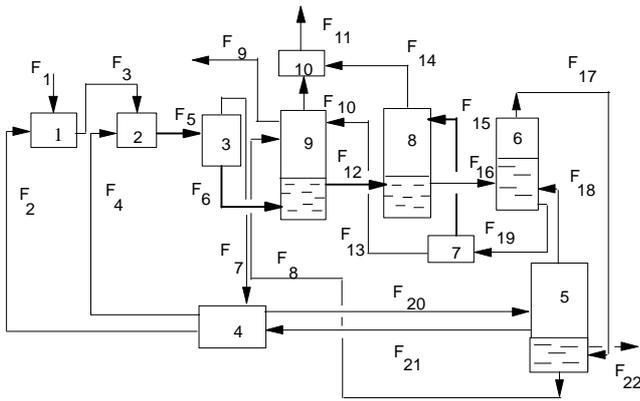
Fig. 3. Structure of a subsystem of a plant for production of ammonia ( $\text{NH}_3$ )
