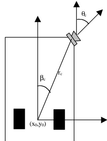
Fig.2 : Sensor's configuration
