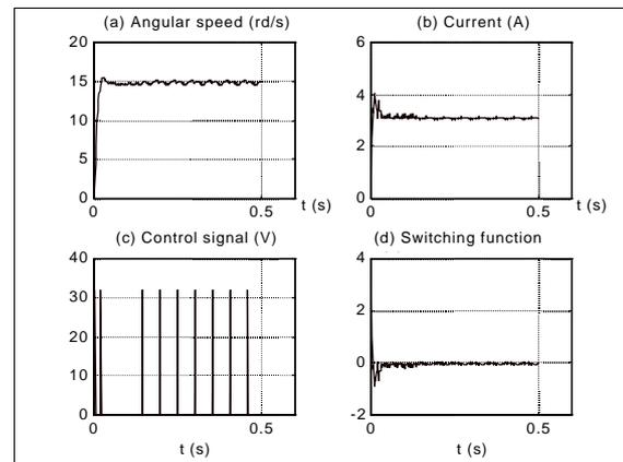
Fig.4. System response at  $E = 250$  W/m<sup>2</sup> and  $I_R = 3.2$  A
