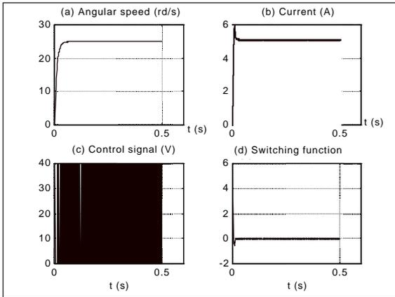
Fig.5. System response at  $E=400\text{w/m}^2$  and  $I_R=5.2\text{A}$
