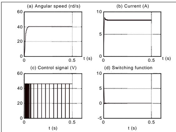
Fig.6. System response at  $E=650\text{w/m}^2$  and  $I_R=8.4\text{A}$
