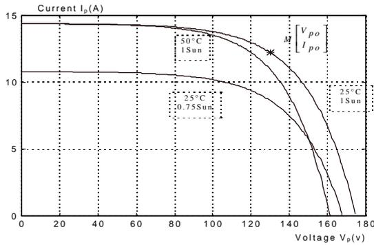
Fig.1. PV generator current-voltage characteristics
