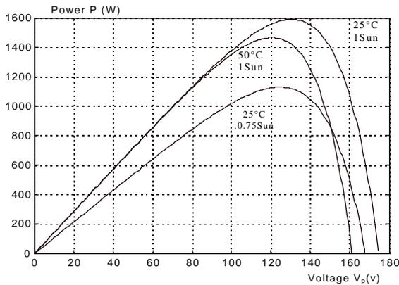
Fig.2. PV generator power-voltage characteristics
