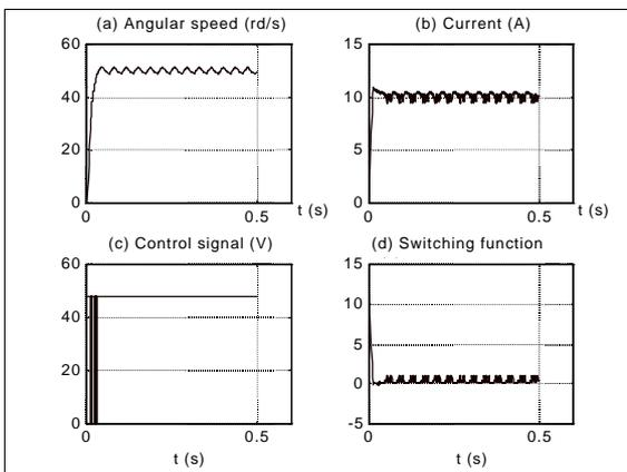
Fig.7. System response at  $E=800\text{w/m}^2$  and  $I_R=10.1\text{A}$
