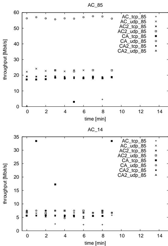
Figure 2:  $A \leftrightarrow C$  tcp and udp measurements.
