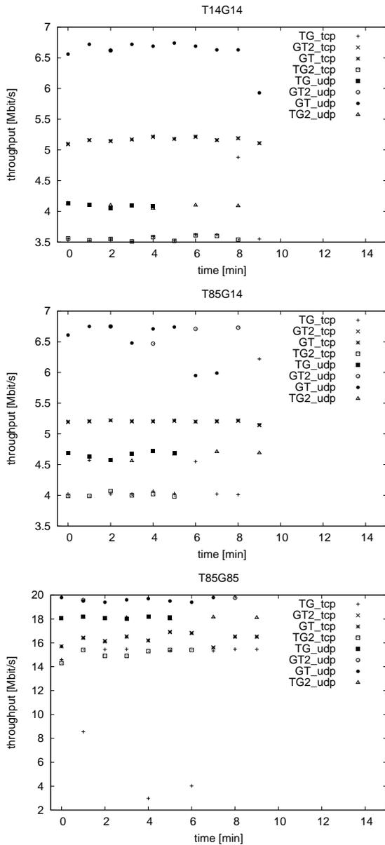
Figure 7: Measurements between two nodes both utilizing 14 Mbps devices, 85 Mbps devices or one node utilizing a 14 Mbps device and the other utilizing a 85 Mbps device.
