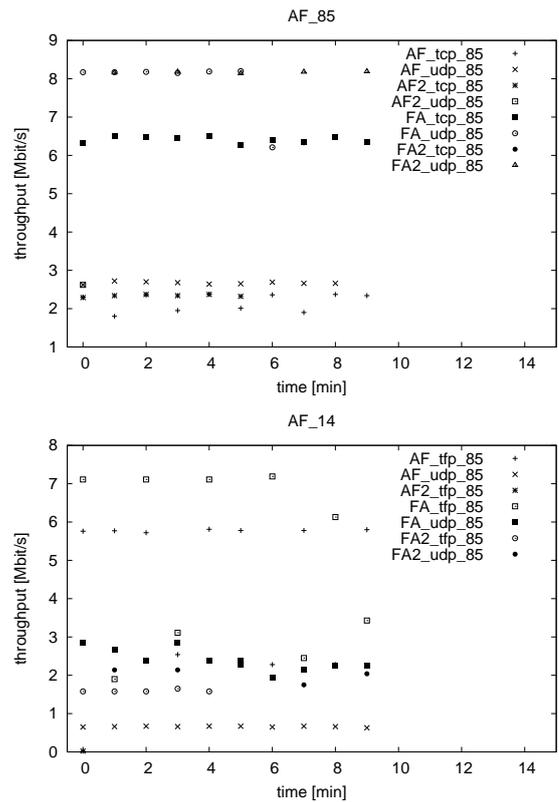
Figure 4:  $A \leftrightarrow F$  tcp and udp measurements.
