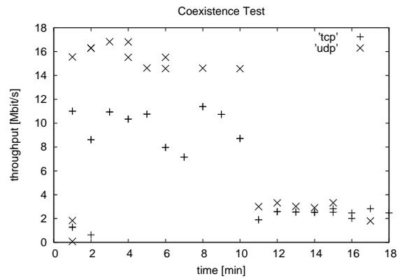
Figure 6: Network coexistence test. Notice that the the lower rate devices “freeze” until the higher rate traffic is finished.
