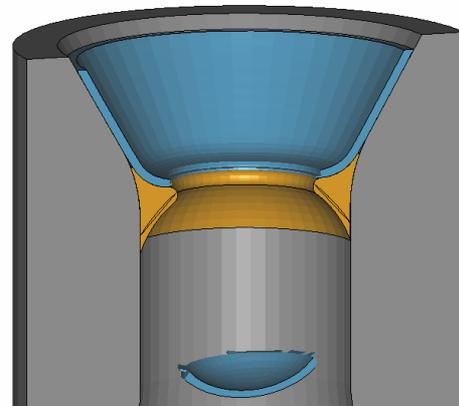
Fig.10 Cap forming from the diaphragm
