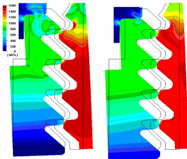
Fig.6 The effective stress threaded assembly for sixth and eighth variants
