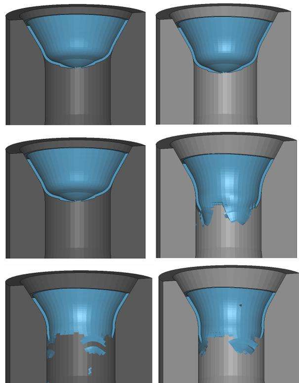
Fig.8 Breaking modes of free diaphragm
