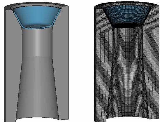
Fig.7 Nozzle – diaphragm assembly
