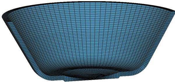
Fig.9 Detail of nozzle – diaphragm assembly
