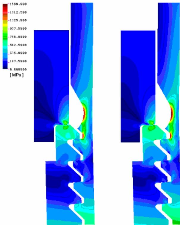
Fig.5 The effective stress threaded assembly for first and second variants
