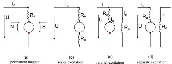
Fig. 2 Equivalent electrical circuits of dc electrical machines for four different kinds of excitation
