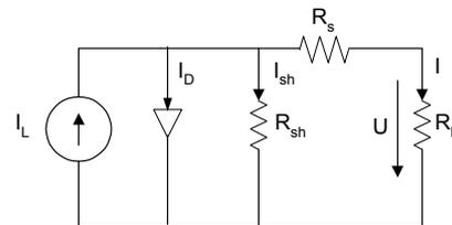
Fig. 1 Equivalent electrical circuit of a solar unit.
