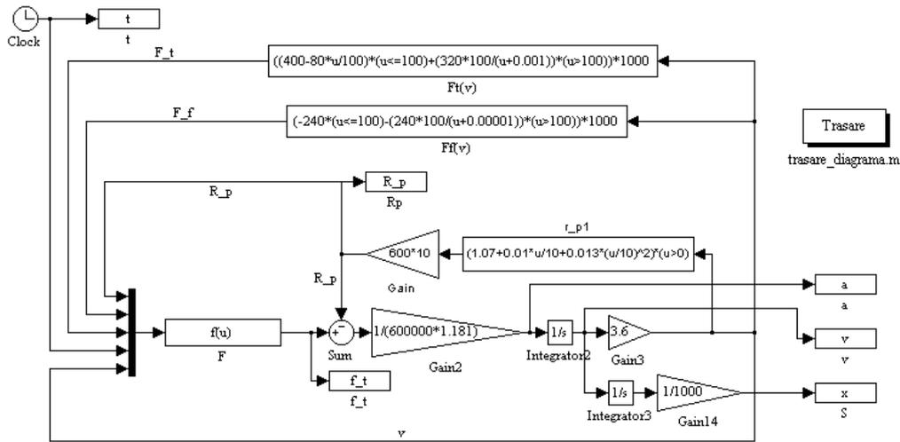
Fig.6 SIMULINK model used for running diagrams drawing
