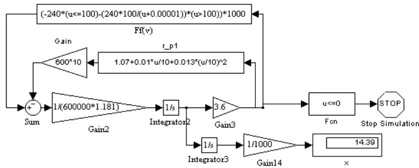
Fig.8 SIMULINK model used establishment of braking distance
