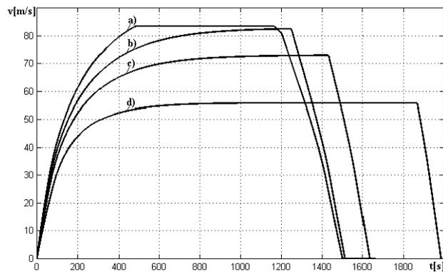
Fig.9 Speed diagram for different values of train resistance (m=600 t)
