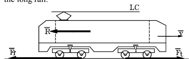
Fig.1 External forces which they establish the movement
