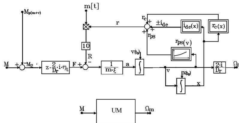
Fig.2 Structural diagram and mask block of useful movement
