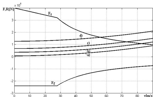
Fig.5 Traction and braking characteristics and 4 values of train resistance of ETR 500 italian high speed train resistance, m=600 t
