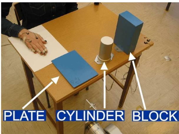
Fig 1. Objects used in the experiment and subject's hand with Optotrak markers
