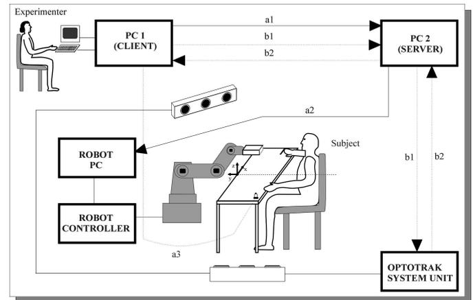
Fig 2. Block scheme of the experimental set-up. After the subject presses the pushbutton, the object is transferred into a randomly selected initial position and the OPTOTRAK starts to collect the data. After three seconds, the subject is informed by an audio signal to start grasping. In the case of perturbation, the robot moved the object into a new pose 0.3s after the issued audio signal.
