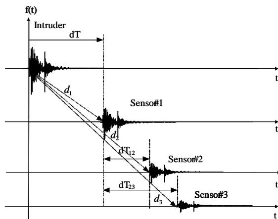
Figure 3: Intruder initiated sound waves with respect to sensors and hub unit
