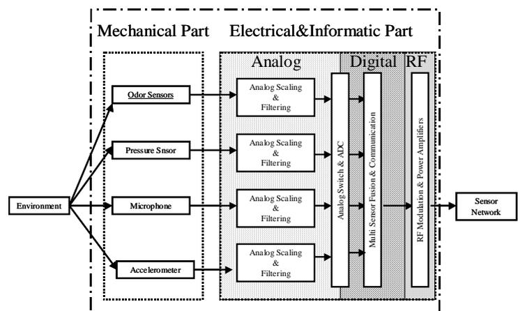
Figure 2: Structural diagram of proposed sensor node.
