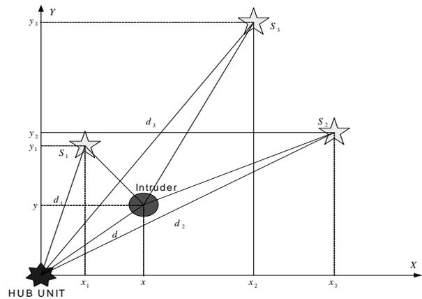
Figure 2: Configuration and definitions for intruder, sensors and hub unit
