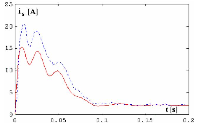
Fig. 5.  $i_s$  computed with the help of the experimental values (blue) and of the simulated ones (red).
