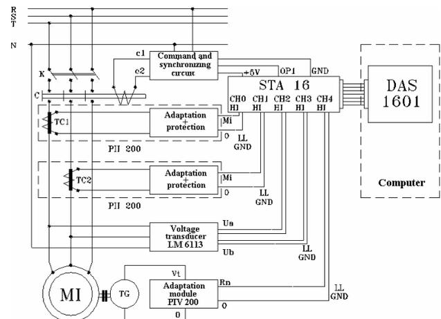
Fig. 2. Connections scheme.
