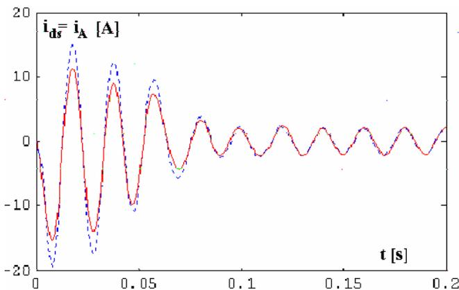
Fig. 3. Components  $i_{ds}$  determined experimentally (blue) and by simulation (red).
