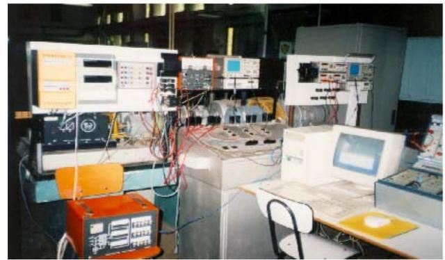
Fig. 1. General view of the computerized micro-bench for induction machines tests.
