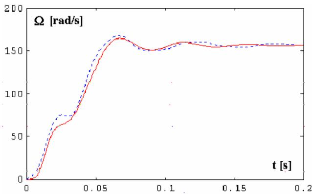
Fig. 7. Angular speeds determined experimentally (blue) and by simulation (red).
