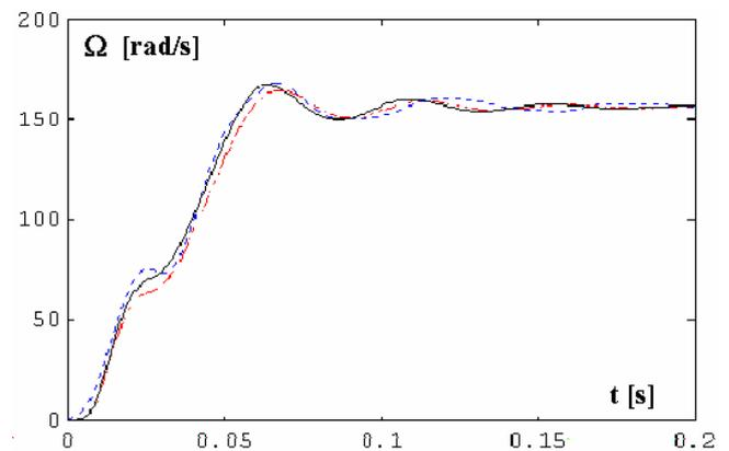
Fig. 9. Angular speed determined experimentally (blue), by simulating with parameters determined classically (red) and by simulation with parameters resulted by optimization (black).
