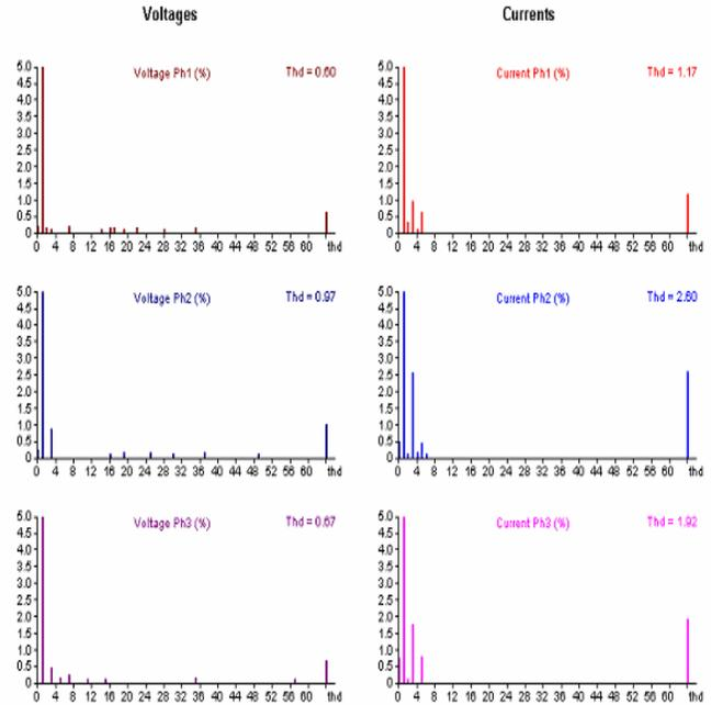
Fig.6. Total harmonic distortion in the arc stable phase
