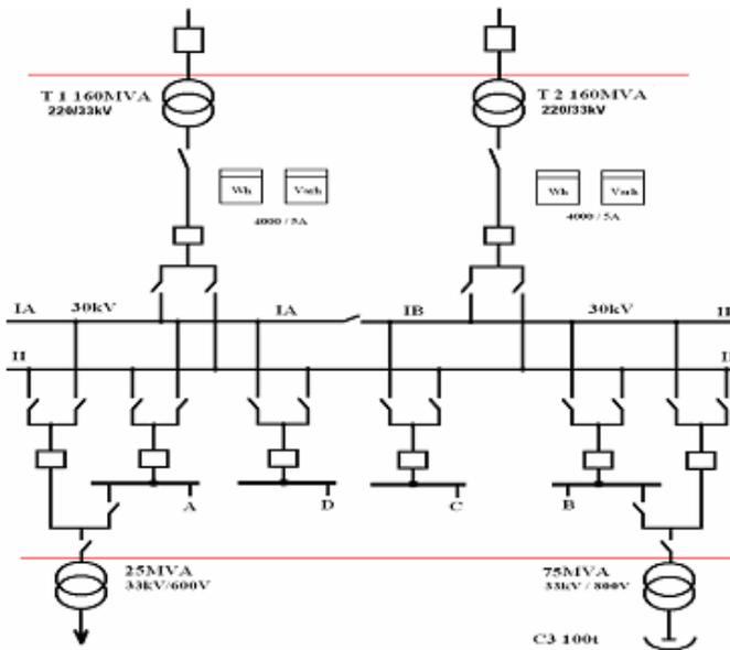
Fig.2. Electrical power supply networks
