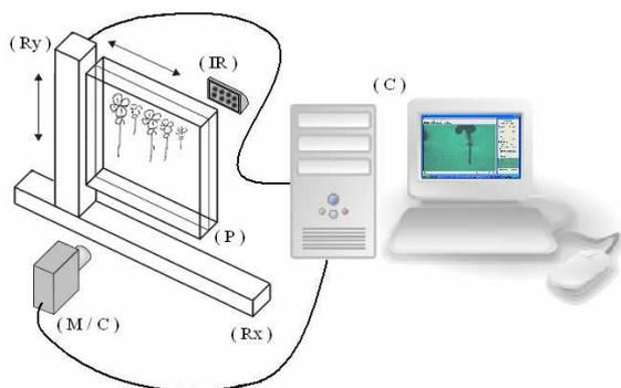
**Fig.1.** Schematic diagram illustrating structure of the hardware component of the ROGO1 platform. An infra red illuminator supplies the video imaging light. A sequence of three time lapse records with 800ms interval is grabbed before each movement of the robot arm. (C) :Controlling computer, (IR) : Infra red light source, (Ry) : y axis of the robot arm, (M / C) : Microscope/Camera unit, (Rx) : x-axis of the robot arm, (P) : Petri dish containing growing seedlings
