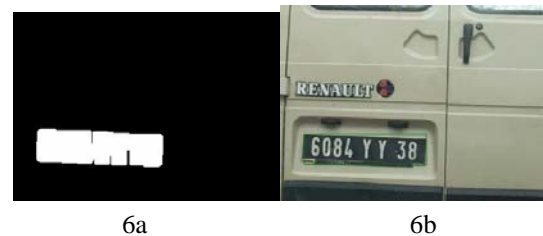
Figure 6a Result of applying conditions like area, bounding box and aspect ratio. 6b shows the final plate area detected in the image within a green rectangle.
