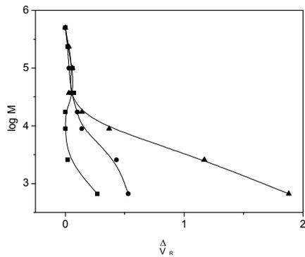
**Figure 6.** Dependence of  $\Delta V_R$  on molar mass of polystyrene probes in THF (▲) C-18 (●) C-8; and (■) C-4 alkyl bonded phases.
