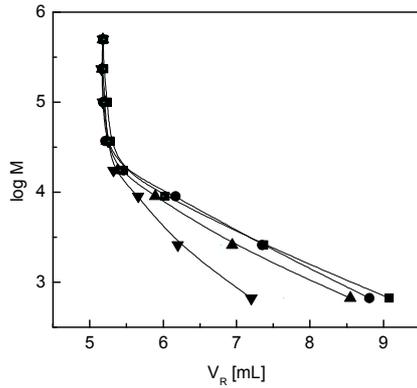
**Figure 4.** Dependences of retention volume of polystyrenes in THF eluent on molar mass of probe. (■) bare silica gel; (●) C-4; (▲) C-8; (▼) C-18 alkyl bonded phases.
