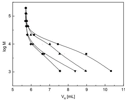
**Figure 5.** Dependences of retention volume of dextrans in methanol/water 20/80 wt./wt. eluent on molar mass of probe. (■) bare silica gel, (▲) C-4; (▼) C-8; (◆) C-18 alkyl bonded phases.
