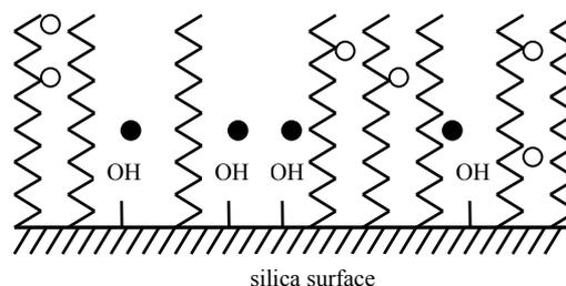
**Figure 2.** Schematic representation of adsorption (●) and enthalpic partition (○) of low molar mass analytes within the alkyl bonded phase.
