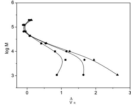
**Figure 7.** Dependence of  $\Delta V_R$  on molar mass of dextran probes in methanol/water 20/80 wt./wt. eluent (▲) C-18; (●) C-8; and (■) C-4 alkyl bonded phases.
