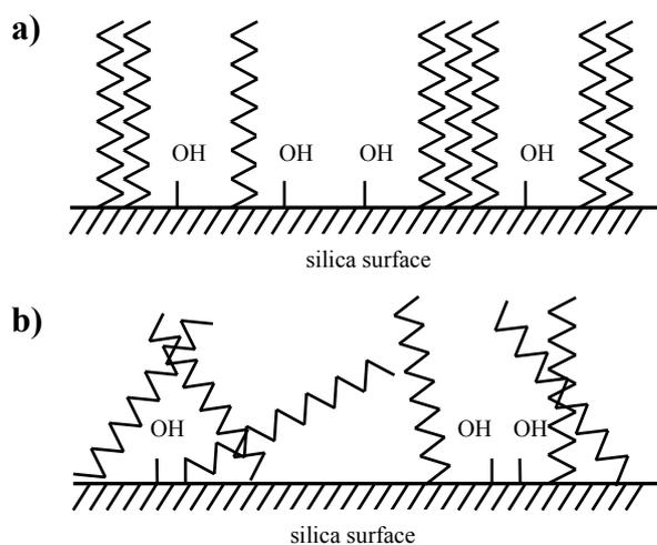
**Figure 1.** Schematic representation of the alkyl bonded silica gel HPLC column packing
