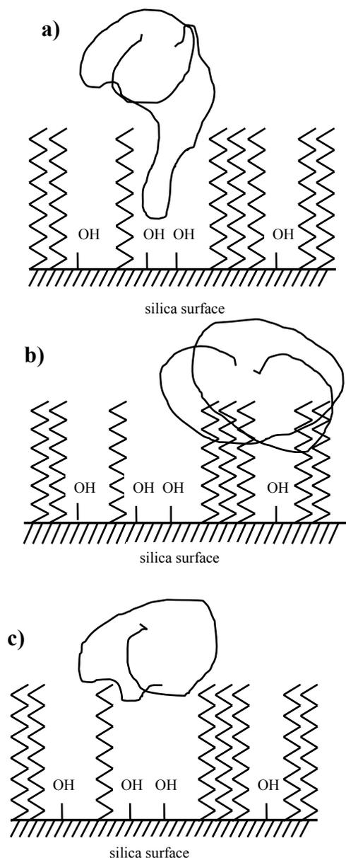
**Figure 3.** Schematic representation of adsorption (a), and enthalpic partition (b) of polymer coil onto/within the alkyl bonded silica gel HPLC column packing. No attractive interaction between polymer coils and column packing is present in the case 3c.
