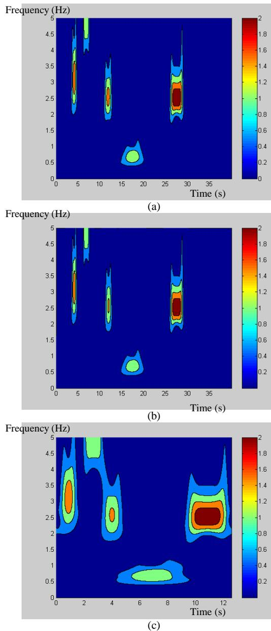
Fig. 4. The pattern of high amplitude events produced by the *S*-transform for T1: (a) The original signal, (b) The identified fatigue damaging events in WBE, (c) The shortened loading
