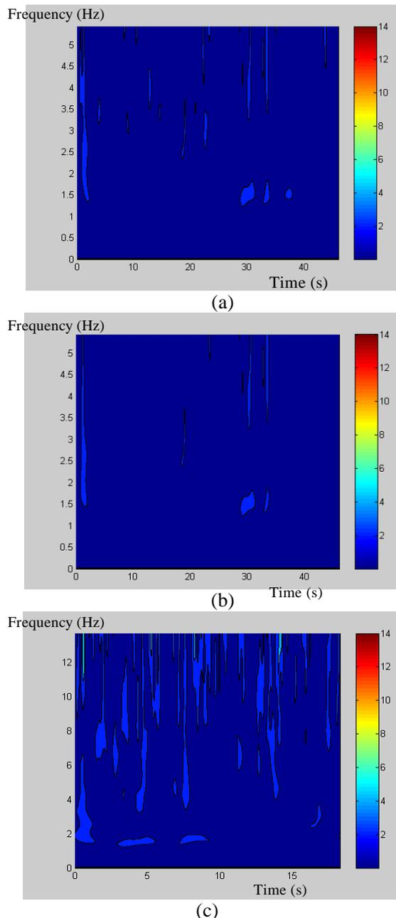
Fig. 5. The pattern of high amplitude events produced by the  $S$ -transform for T2: (a) The original signal, (b) The identified fatigue damaging events in WBE, (c) The shortened loading
