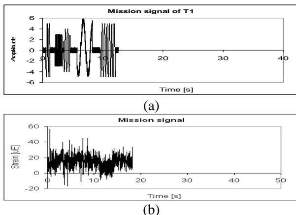
Fig. 3. The shortened loadings produced using the WBE algorithm: (a) The 12.5-second T1 loading, (b) The 19-second T2 loading
