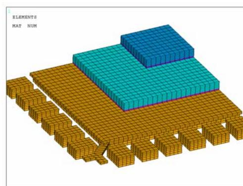
Fig. 2 Meshed Quarter Model for QFN Package
