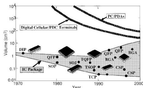
Fig. 1 Trend of miniaturization of IC package
