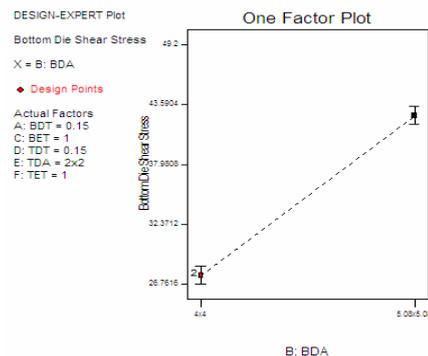
Fig. 6 One factor plot for Bottom Die Area
