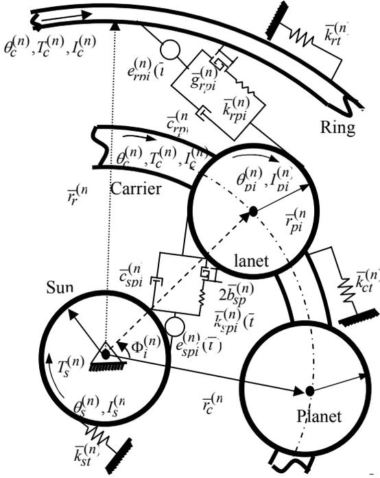
Fig. 2 Dynamic model of a single-stage
