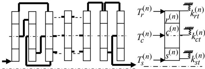
Fig. 1 Stick diagram, a) Multi deck compound planetary gear set. b) the  $n$ th deck external applied torques and torsional constraints
