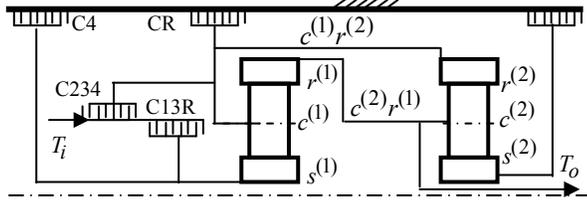
Fig. 3 Two deck planetary set.
