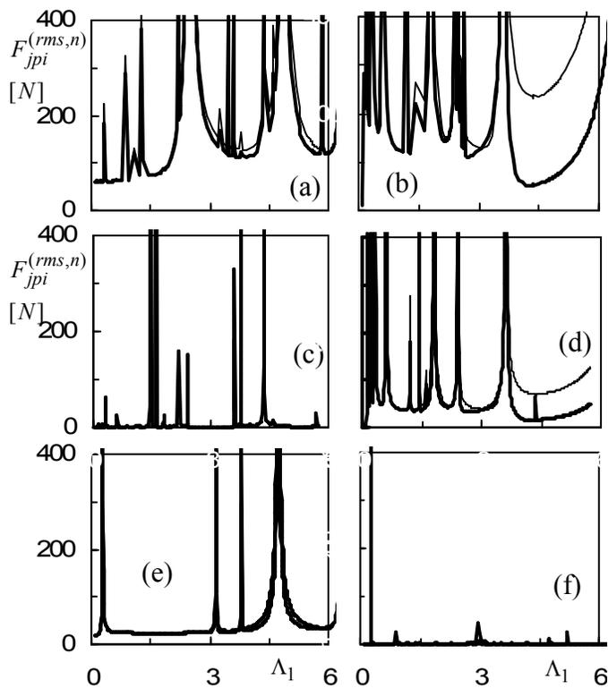
Fig. 5, rms mesh force response. (a), (c) and (d) for deck-1 meshes. (b), (d) and (f) for deck-2 meshes. (-) sun/planet meshes, (~) ring/planet meshes.
