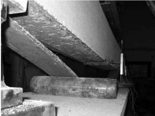
Fig 7. Failure mode of the R-2W – FRP debonding
