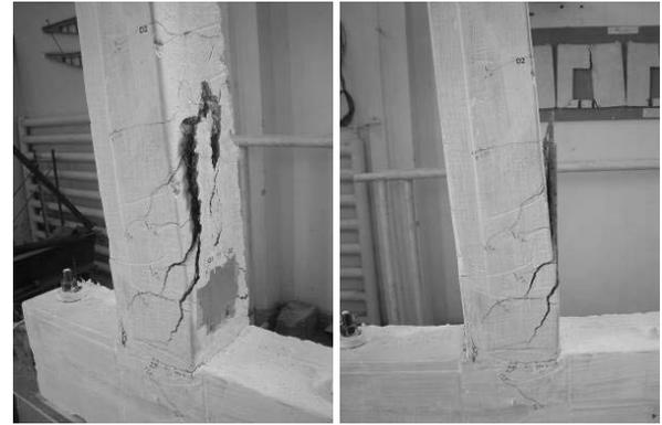
Fig 13. Failure mode of the C3M-BM-AF specimen
