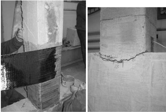
Fig 16. Strengthening and failure detail of the C1C-CW-BC specimen
