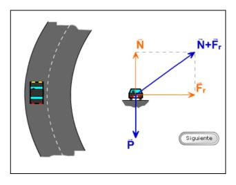
In Fig. 3 above we show an example of the first class, showing forces acting on a car on a curve. In Fig. 4 below we show and interactive example of the method of energy conservation applied to a problem in point Dynamics.
