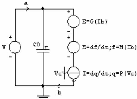
Fig. 5. Controlled source implementation of the first nonlinear circuit model
