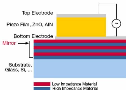
Fig. 1 Solidly mounted resonator (SMR)
