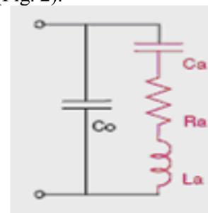
Fig. 2 Butterworth-Van Dyke circuit
