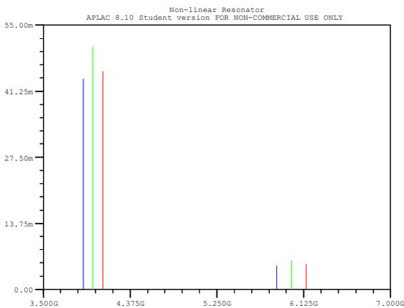
Fig. 7. Intermodulation products for V=5V, first model
