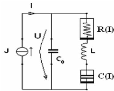
Fig.4. Linear parametric model of a quartz resonator
