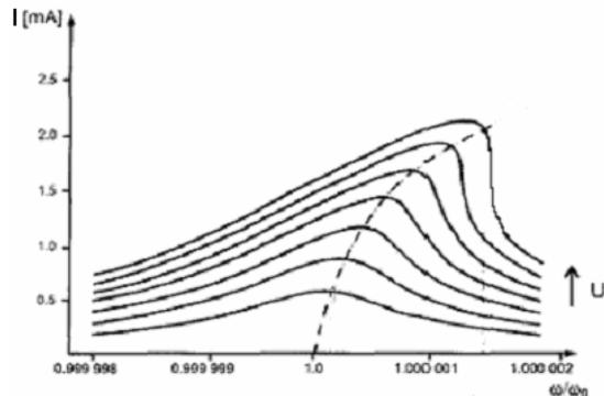
Fig. 3. Frequency characteristics of a quartz resonator (I- resonator current, U- excitation voltage)
