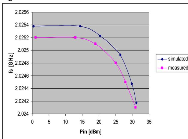
Fig. 11. The dependence of the series resonance frequency on the incident power
