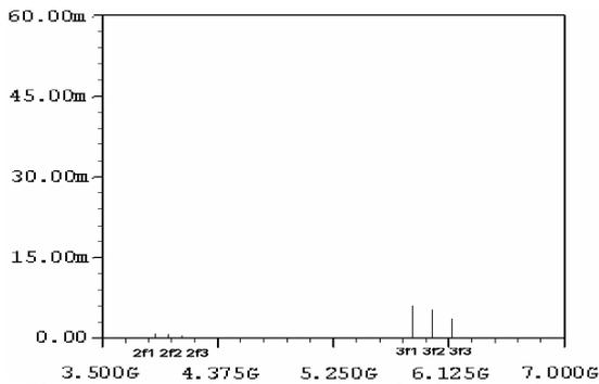
Fig. 10. Intermodulation products for the second model with modified inductor characteristic
