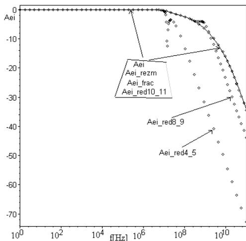
Fig. 3. Bode characteristics: *Aei*, *Aei\_rezm*, *Aei\_frac*, *Aei\_red10\_11*, *Aei\_red8\_9*, and *Aei\_red4\_5*.
