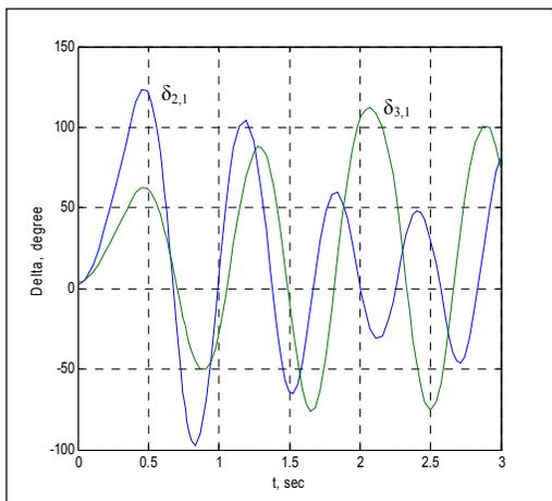
Fig. 3 Differences of rotor angle for generators 2 and 3 corresponds to generator 1.
