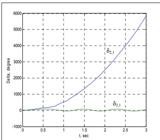
Fig. 4. Differences of rotor angle during unstable condition
