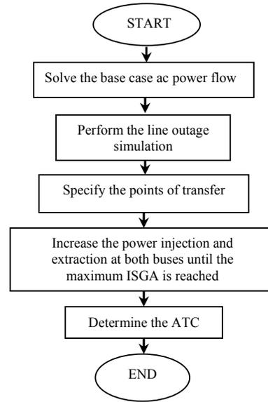
Fig. 1 Flowchart of ATC determination using recursive AC power flow method
