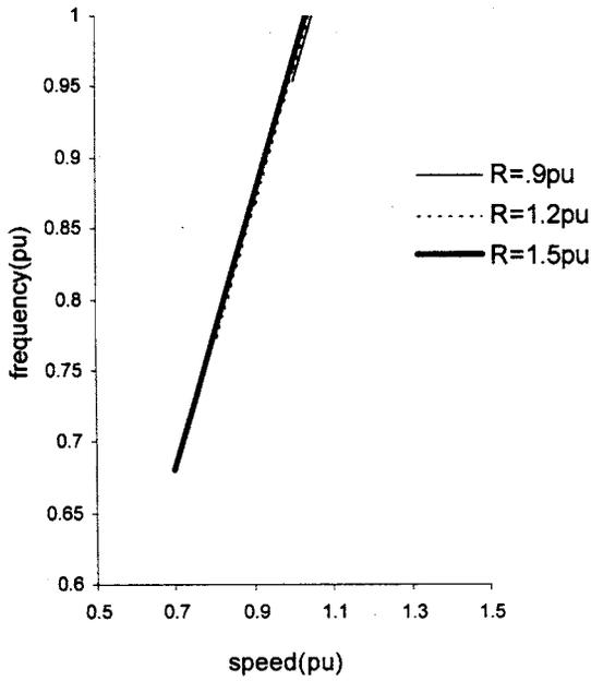
Fig. 7 Variation of frequency with operating speed, C=1pu
