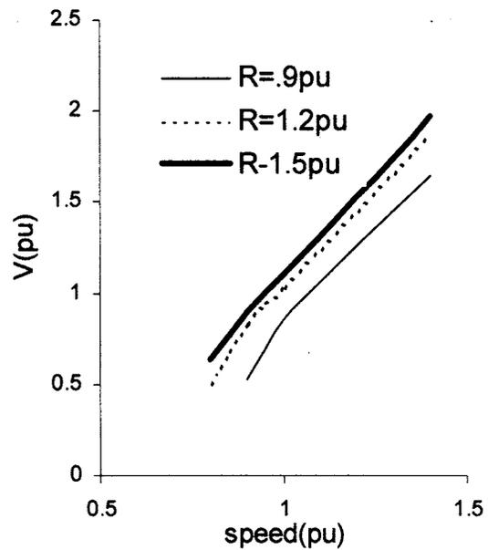
Fig. 6 Variation of voltage with operating speed,  $C=1pu$
