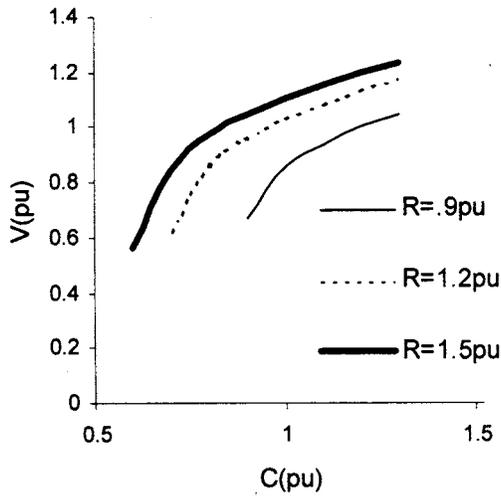
Fig. 3 Variation of voltage with excitation capacitance,  $b=1pu$
