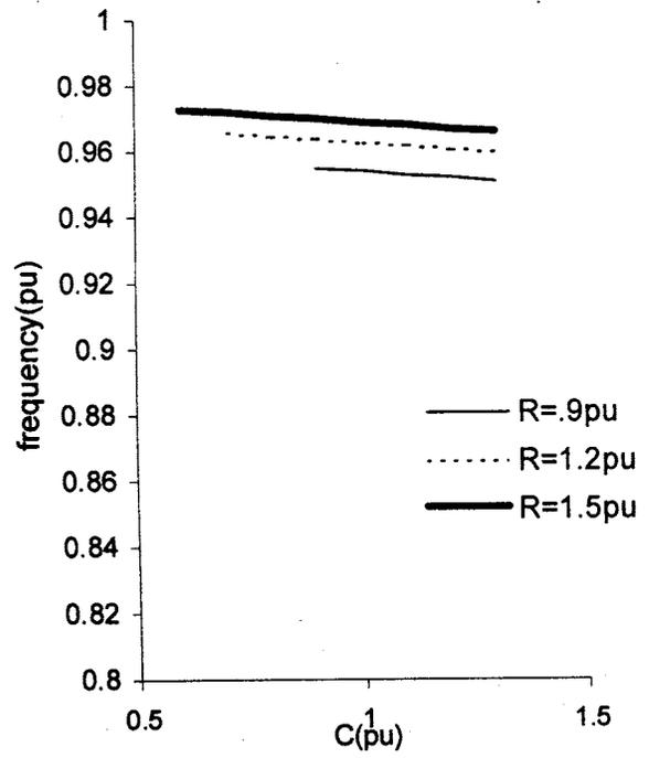
Fig. 5 Variation of frequency with excitation capacitance,  $b=1pu$
