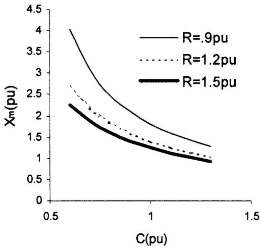
Fig. 4 Variation of magnetizing reactance with excitation capacitance,  $b=1pu$
