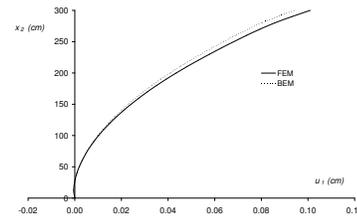
Fig. 6. Variation of the horizontal component of displacement vector on line AK
