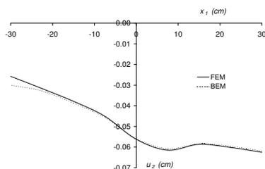
Fig. 11. Variation of the vertical component of displacement vector on line KC
