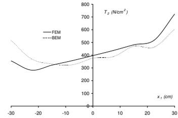
Fig. 5. Variation of the vertical component of surface traction vector on line AB
