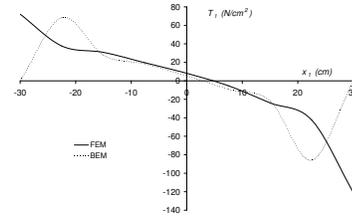
Fig. 4. Variation of the horizontal component of surface traction vector on line AB
