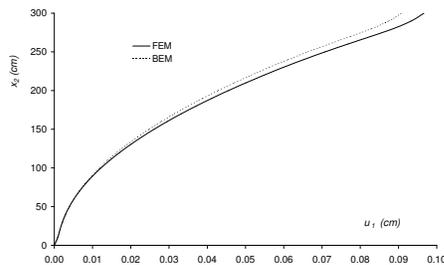
Fig. 8. Variation of the horizontal component of displacement vector on line CB
