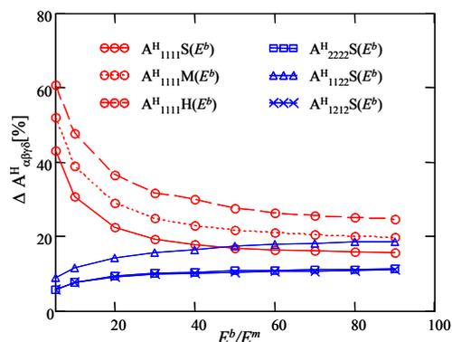
Figure 17  $\Delta A^H_{\alpha\beta\gamma\delta}$  increment of in-plane stiffness for strengthened masonry in comparison with un-strengthened one.
