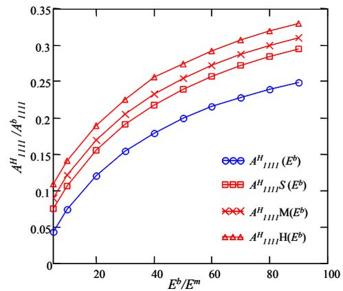
Figure 13  $A^H_{1111}$  comparison between un-strengthened and strengthened masonry.
