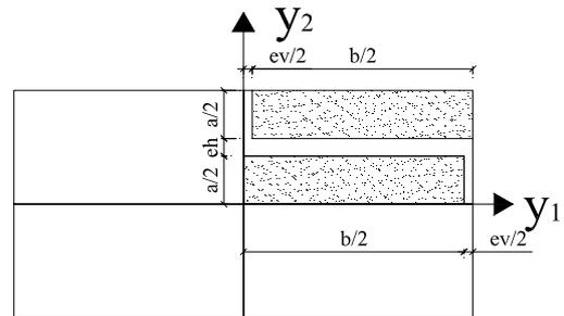
Figure 6 From the elementary cell  $Y$  (a) to  $Y/4$  (b) for F.E.M. homogenisation procedure.
