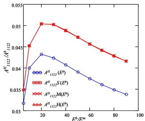
Figure 15  $A^H_{1122}$  comparison between un-strengthened and strengthened masonry.
