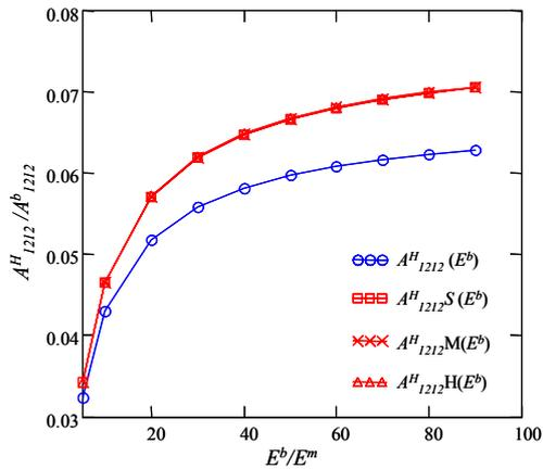
Figure 16  $A^H_{1212}$  comparison between un-strengthened and strengthened masonry.
