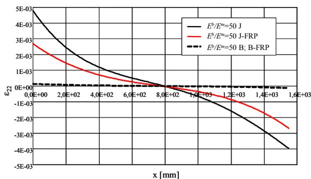
Figure 20  $\varepsilon_{22}$  along layers  $B$  and  $J$ , for  $\xi^{-1}=50$  ratio, for 2D heterogeneous model and 2D homogenised FRP model evaluated by numerical homogenisation procedure.
