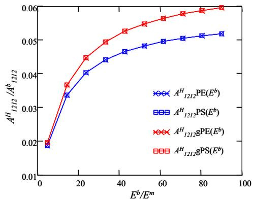
Figure 5 Trend of membrane modulus  $A^H_{1212}$ .
