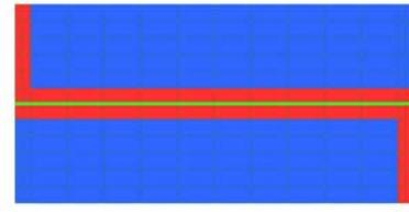
Figure 8  $Y/4$  elementary cell meshing of strengthened masonry.
