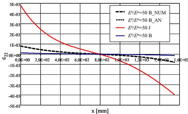
Figure 19  $\varepsilon_{22}$  in layers  $B$  and  $J$ , in 2D heterogeneous model and 2D homogenised model, evaluated by analytical and numerical homogenisation procedure.
