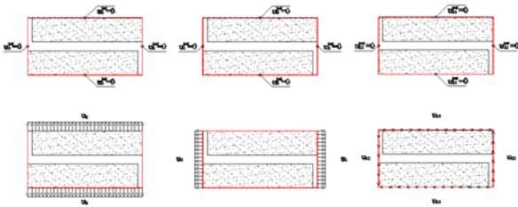
Figure 7 Displacement conditions on 2D elementary cell
