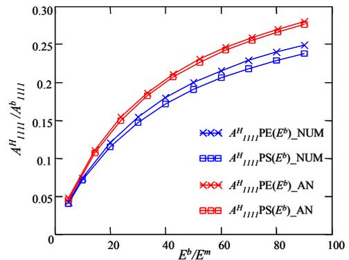
Figure 9 Trend of membrane modulus  $A^H_{1111}$ .
