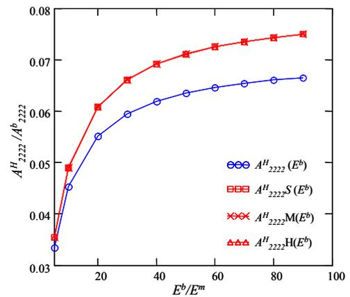
Figure 14  $A^H_{2222}$  comparison between un-strengthened and strengthened masonry.
