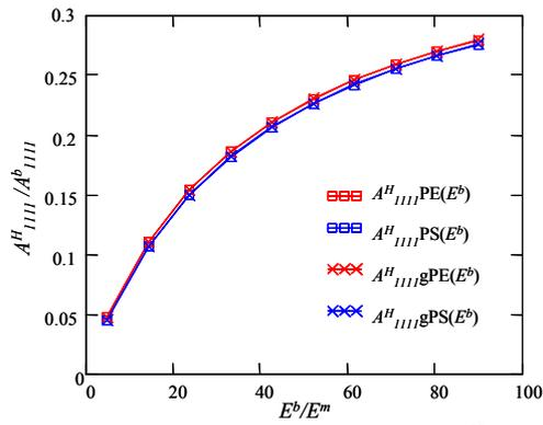
Figure 2 Trend of membrane modulus  $A^H_{1111}$ .
