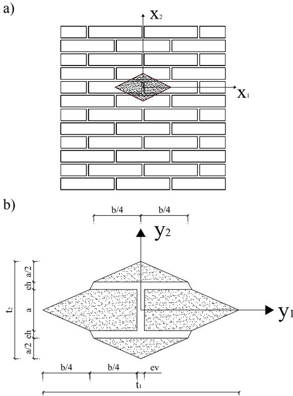
Figure 1 The elementary cell: Y-REV
