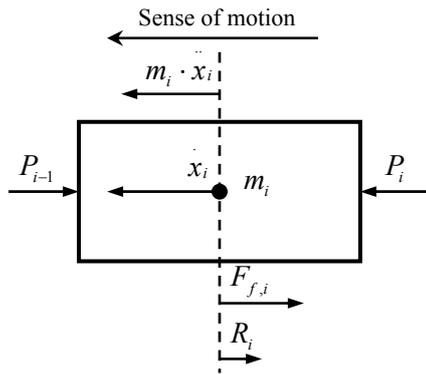
Fig. 2. Forces acting on a vehicle within the train during braking.
