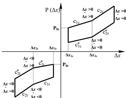
Fig. 3. General elastic characteristics of shock (index c) and traction (index t) apparatus.
