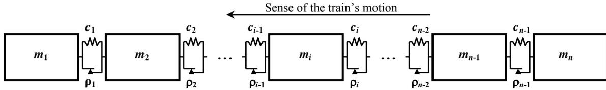
Fig. 1. Mechanical model of the train.
