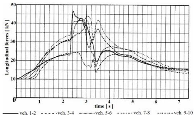
**Fig. 5. Evolution of longitudinal dynamic forces within the train body during emergency braking action (10 identical vehicles of 30 t mass each).**
