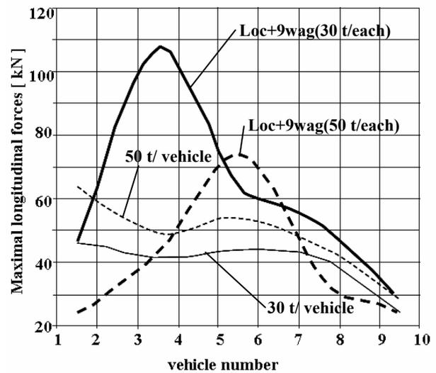
**Fig. 8. Assessment of maximal longitudinal forces along the 10 vehicles train during an emergency braking action from 250 km/h (thick lines – locomotive+9 identical passenger wagons, thin lines – 10 identical vehicles).**
