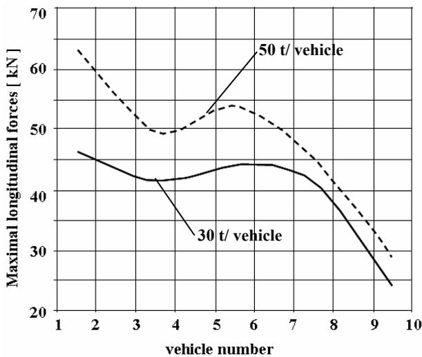
**Fig. 7. Assessment of maximal longitudinal forces along the 10 identical vehicles train during an emergency braking action from 250 km/h.**
