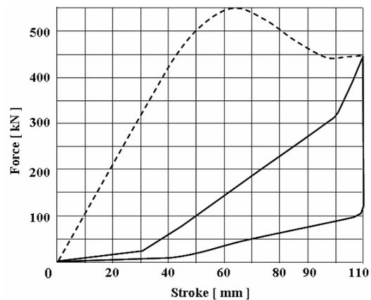
Fig. 4. Theoretical characteristic diagrams of the lateral buffers for passenger vehicle ( ——— static; - - - - dynamic ).
