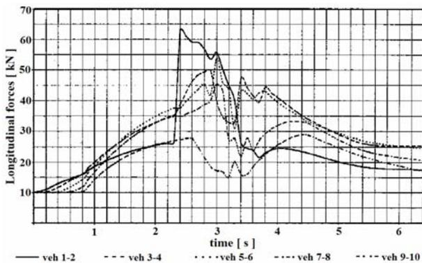
**Fig. 6. Evolution of longitudinal dynamic forces within the train body during emergency braking action (10 identical vehicles of 50 t mass each).**
