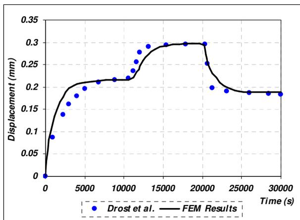
Fig. 3: Validation of the model with Drost's Experimental Data
