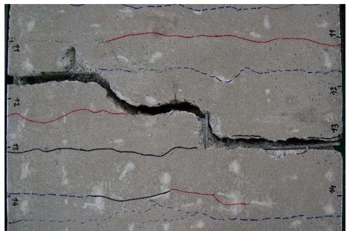
Fig. 10 Reinforced concrete slab No. 4. The marked cracks and the final crack between the cross-sections No.12 and 13.
