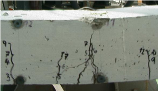
Fig. 4 Reinforced concrete beam No. 3. The marked cracks and the final crack in the cross-section No. 11
