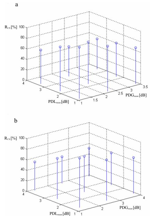
Fig4. Impact of  $PDL_{mean}$  and  $PDG_{mean}$  on  $R_{cx}$  ratio; n=150 (a), n=200 (b)
