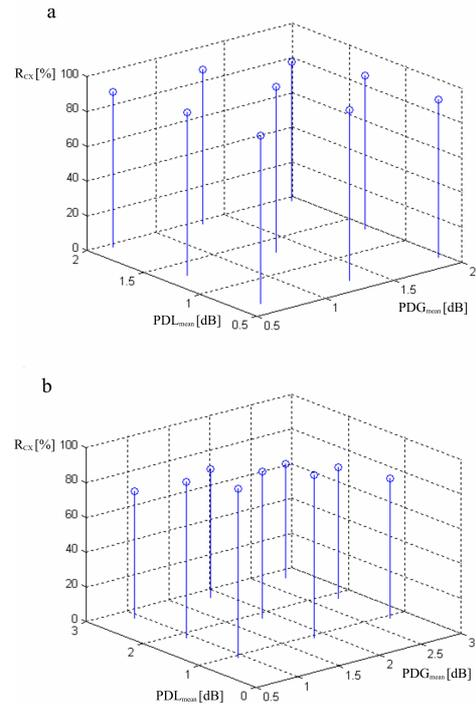
Fig. 3. Impact of  $PDL_{mean}$  and  $PDG_{mean}$  on  $R_{cx}$  ratio; n=50 (a), n=100 (b)
