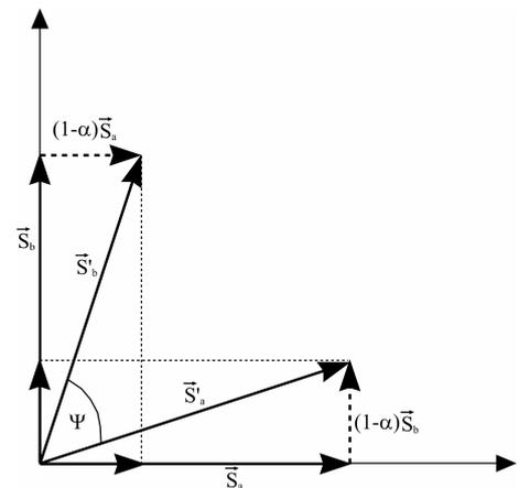
Fig. 1. Loss of orthogonality between SOPs vectors
