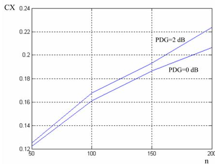
Fig. 2. Crosstalk evolution as a function of number of birefringence segments n; PDL=0.2 dB
