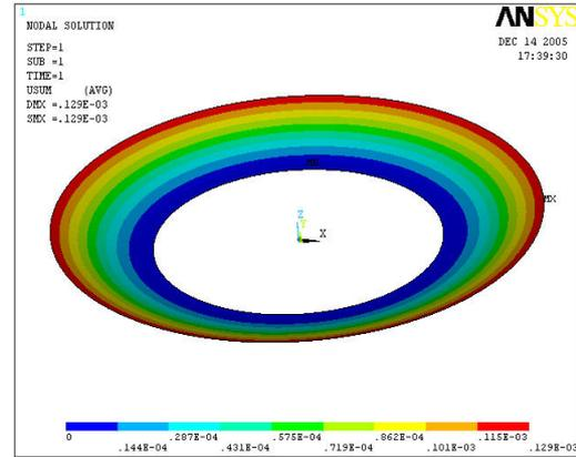
Fig.6 The simulation deformation of single and multi-slices
