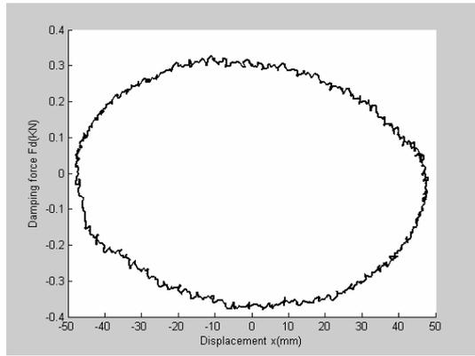
Fig.8 The indicator diagram of damper with single and multi-slices
