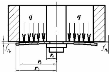
Superposition throttle slice of unequal thickness could be taken as the springs paralleled that have the equal length, but unequal elasticity coefficient. So, the deformations of multi-slices are equal, the forces on multi-slices are unequal. The composition of forces on multi-slices is equal to the total force. According to the bending deformation formula of throttle slice (3), it can be obtained as
