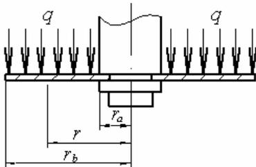
Fig. 1 Mechanics model of elastic throttle slice
