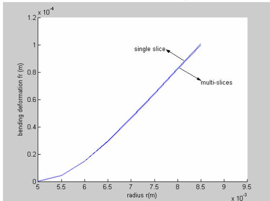
Fig.5 The bending deformation curves of multi-slices and single slice
