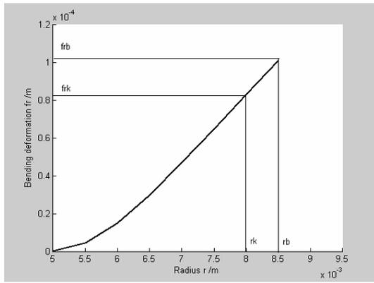
Fig3. The curve of deformation fr Vs. r
