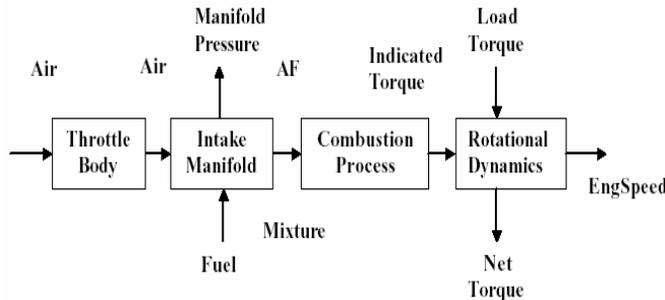
Fig. 2. Engine Model Description
