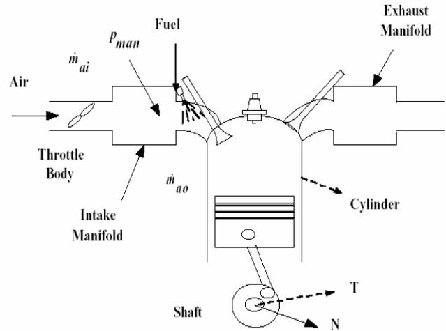
Fig. 1. Schematic Diagram of IC Engine
