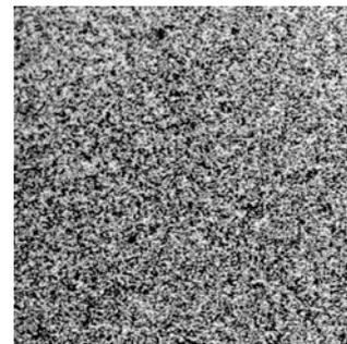
Fig. 1. A typical recorded speckle pattern.
