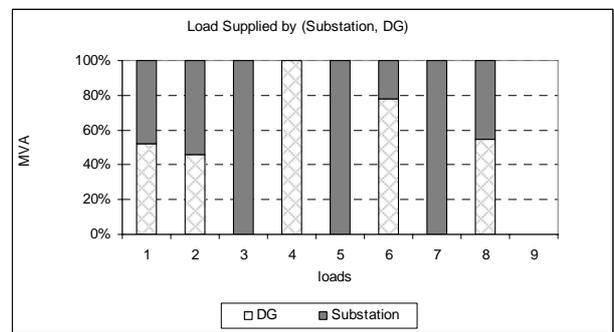
Fig.6 Load Supplied by Substation and DG for the DG option
