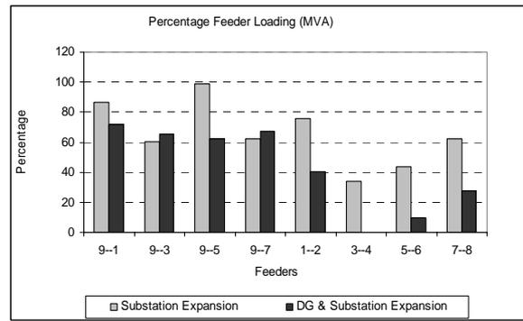
Fig.5 Percentage Feeder Loadings
