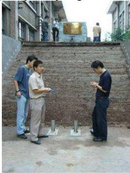
Fig.3 Image of the Physical model to simulate debris flow on hillside
