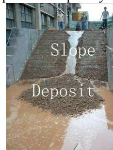
Fig. 11 Landform after occurrence of debris flow
