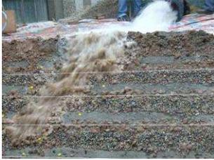
Fig.6 Simulation of heavy rainfall and torrent on slope
