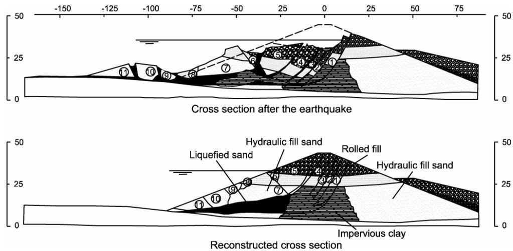
Fig. 1. Geometry of the Lower San Fernando dam after and before the failure in the 1971 earthquake [11]. Dimensions in meters.
