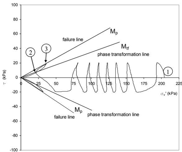
Fig.2. Cyclic shear stress test on saturated loose undrained sand. Stress path, failure and phase transformation lines. (after [14])
