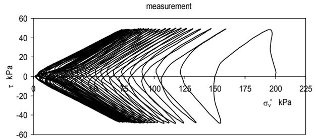
Fig.3. Cyclic shear stress test in dense saturated undrained sand. Stress path (after [14])
