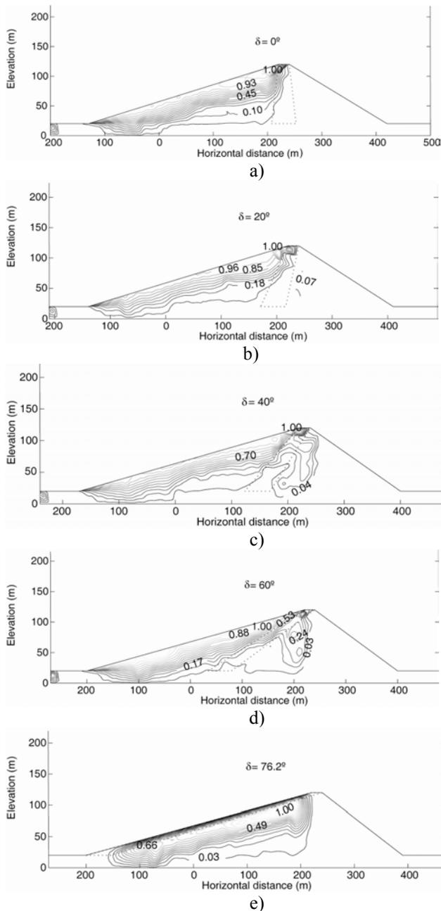
Fig.5. Computed liquefaction degree  $r_u = \Delta p_w / \sigma'_{v0}$  in the dams at the end of the earthquake
