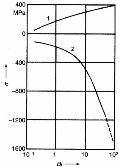
**Fig. 3** Tensile hoop stresses at the core (1) and maximum compressive hoop stresses at the surface (2) for cylinders depending on Biot number  $Bi$ .
