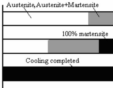
**Fig.1** Relative amounts of microstructural phases present in a steel specimen at the beginning and end of intensive quenching, and at the time when the surface compressive stress reaches its maximum value (see the second tape).
