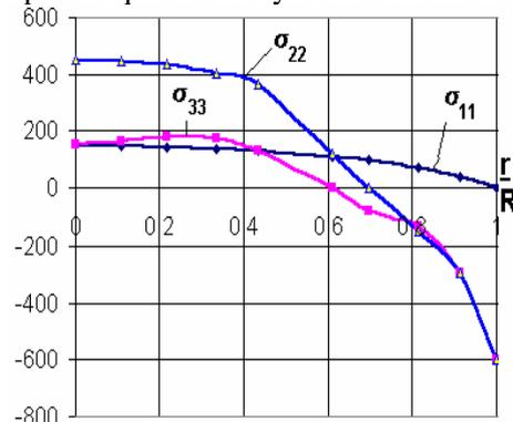
**Fig. 2** The distribution of stresses on the cross section of cylindrical samples of diameter of 6 mm and 60 mm at the time of reaching maximum compressive stresses on the surface. ( $Bi = 7$ ;  $Fo = 0.7$ ); 1 – sample of 6-mm-diameter; 2 – sample of 60-mm-diameter.
