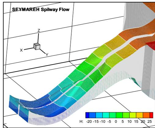
Fi.3, computed water surface elevation , general view (up) close view (down)
