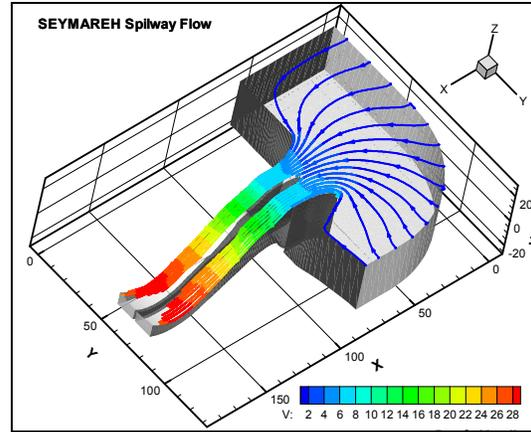
Fig.5, Computed stream lines, general view
