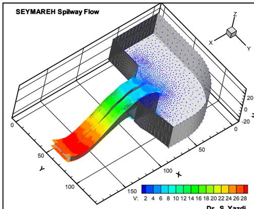
Fig.4, Computed velocity vectors
