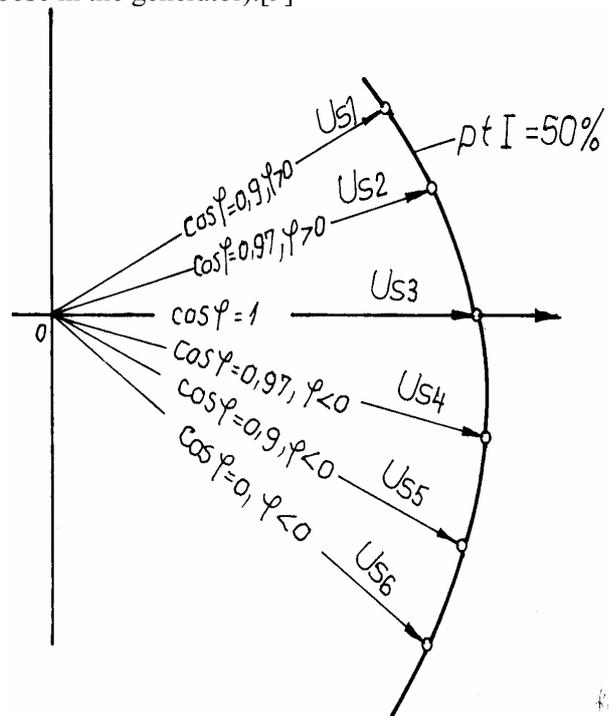
Fig. 3. Hodograph (geometric place of a vector extremity)  $\bar{U} = f(\cos \varphi)$ ,  $I = 50\%$ .
