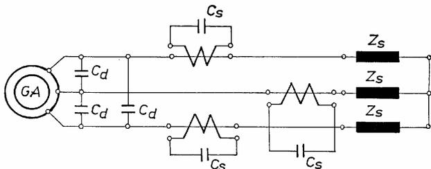
Fig. 8 Schematic diagram of condenser excited induction
