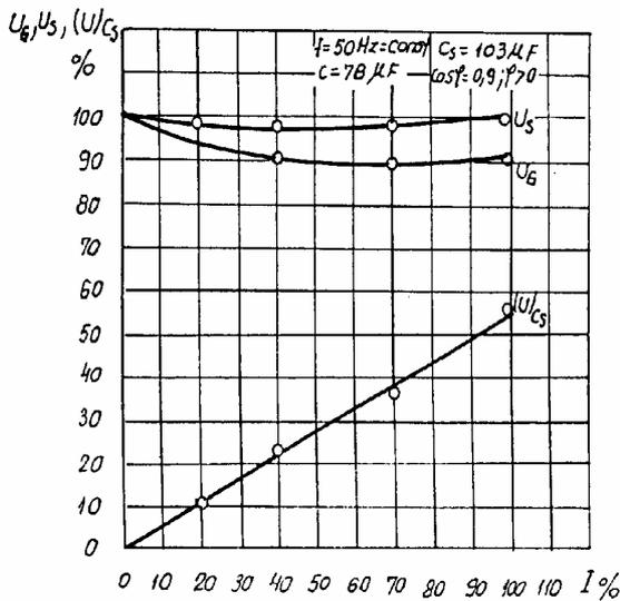
Fig. 7 Voltage  $U_s$ ,  $U_G$ ,  $(U)_{C_s}$  characteristics of compounded induction generator at inductive character load with power factor  $\cos \varphi_s = 0,9$
