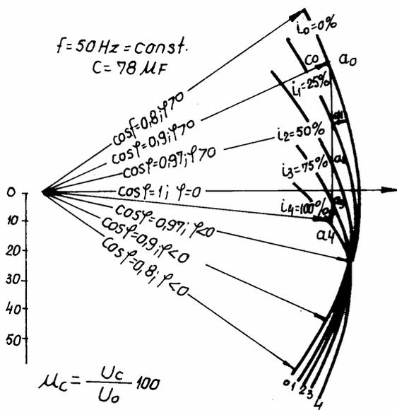
Fig. 4 Hodograph  $\bar{U} = f_k(\cos \varphi)$  for different values of the current  $I_k = const.$
