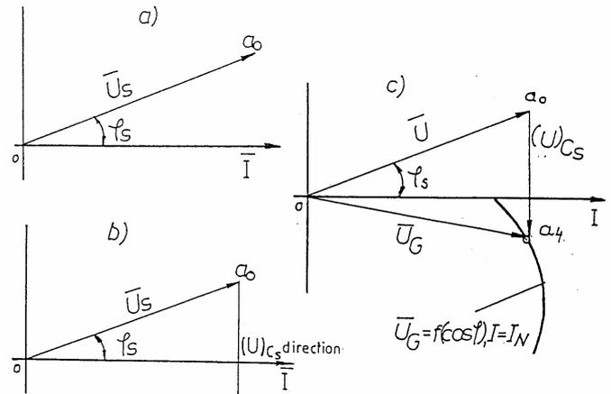
Fig. 5 Graphical determination of the phasor  $(\bar{U})_{C_s}$  on the condenser required for the compensation of voltage lose in the generator.
