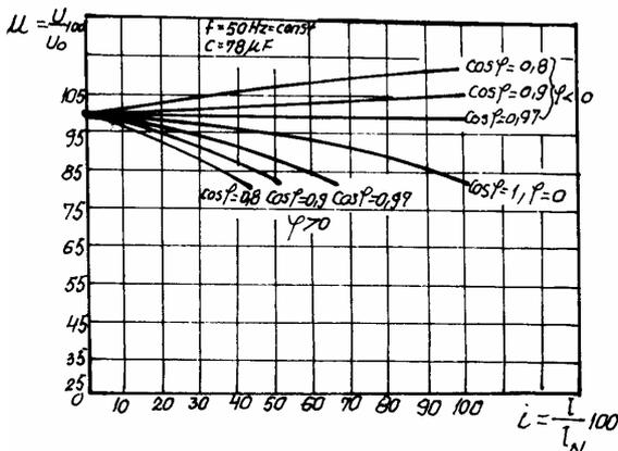
Fig. 2 External characteristic family for the induction generator.
