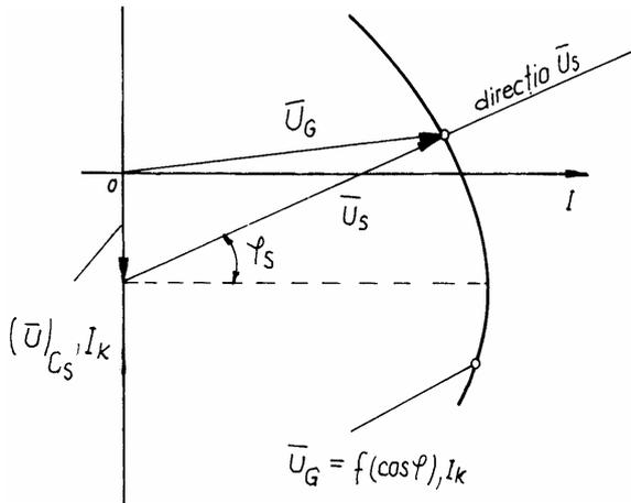
Fig. 6  $\bar{U}_s$  phasor construction for given values of  $C_d$ ,  $C_s$ , and  $I$ .
