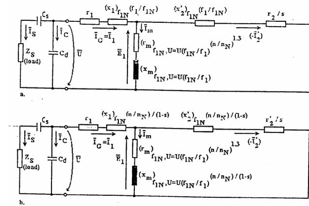
Fig. 9 Compound condenser-excited induction generator
