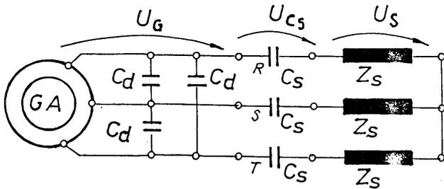
Fig. 1 Schematic diagram of compound induction generator power circuit.
